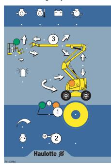
Movements can be controlled when the main energy source malfunctions. There is an electropump unit powered by the starter battery. This unit can be controlled from either the turntable control panel or the platform control panel.
