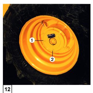
The wheel must be dismantled for checks and drainage. To do so, immobilise the machine and lift using a jack or a hoist.
